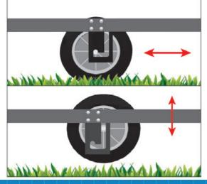
Easily engage wheels to move tool around, disengage to start working.
