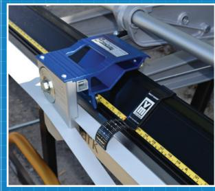
TrimCutter<sup>™</sup> cuts steel, aluminum, copper, and zinc. We use a dual track system with 4 wheels for precise cuts. (Optional Accessories)
